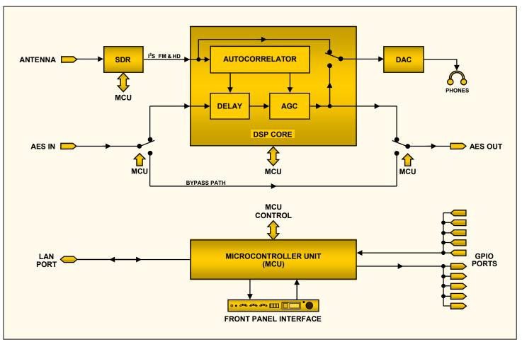
Block Diagram – JUSTIN 808 HD Radio<sup>™</sup> Time Alignment Processor
